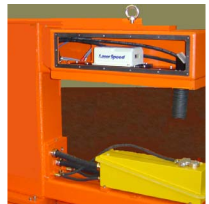
LS8000C, C-frame mounted inside an X-ray Thickness Gauge
