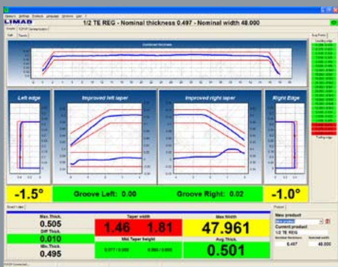
Operators software showing dimensional profiles
