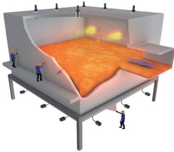
*Obtaining reliable temperature measurement in the melting tank*
