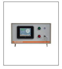
The test chamber is then placed under a vacuum that forces air from any openings within the pack. After returning to an ambient pressure, the dye will penetrate and be evident within the pack should any holes be present.
